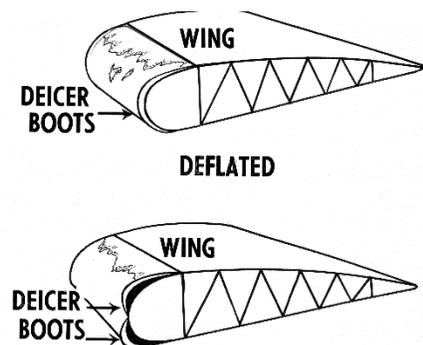
Figure 1: Pneumatic Deicing Boot
