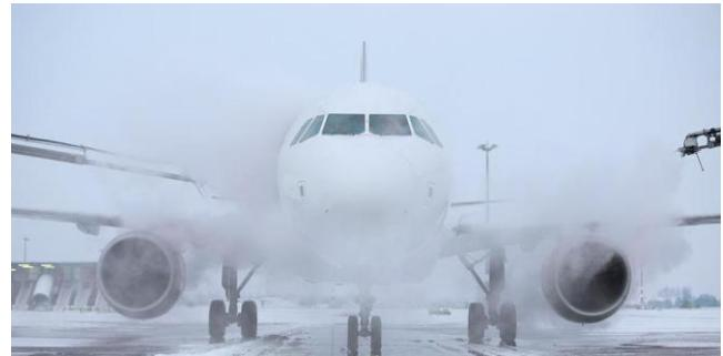
Figure 2: Chemical De-Icing on the Ground
