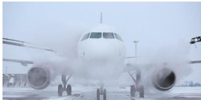
**Figure 2: Chemical De-Icing on the Ground**
