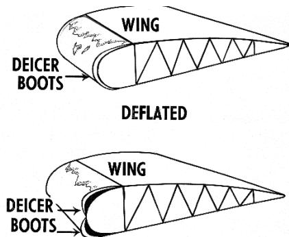
Figure 1: Pneumatic Deicing Boot
